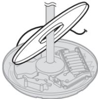
2 Install the batteries in the battery holder.
