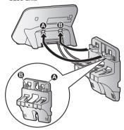
4 Adjust the adaptor to hold the base unit, then push it in the direction of the arrow until it clicks into place.
