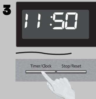
Press **Timer/Clock** to finish setting and the colon (:) will stop blinking.
