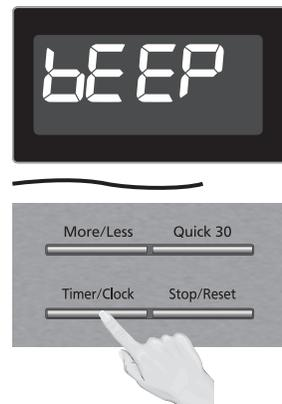
Press **Dial** once, then Press **Timer/Clock** to cycle between the Beep on or Beep off.
