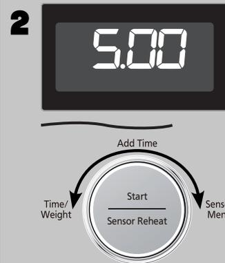
Set cooking time using the **Dial**. P10 (HIGH) and P0 (KEEP WARM) have max. cooking time of 30 minutes. For other power levels, the max. time is 1 hour 30 minutes.
