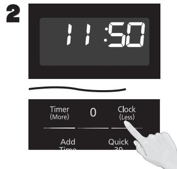
Press **Clock (Less)** to finish setting and the colon (:) will stop blinking.
