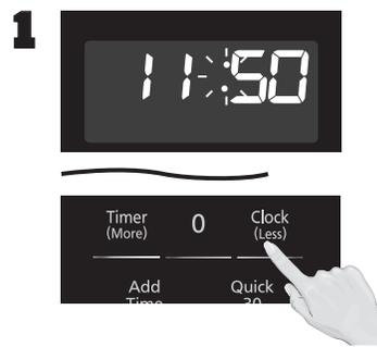
With the oven **NOT** cooking, press **Clock (Less)** once; the colon will blink. Enter time of day using the **Number** pads.
