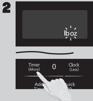
Press **Start** once, then Press **Timer (More)** to cycle between the weight system, Imperial (oz/lb) or Metric (g/kg).
