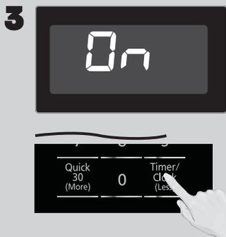
Press **Start** once, then Press **Timer/Clock (Less)** to cycle between the Beep on or Beep off.
