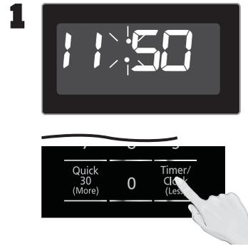
With the oven **NOT** cooking, press **Timer/Clock (Less)** twice; the colon will blink. Enter time of day using the **Number** pads.
