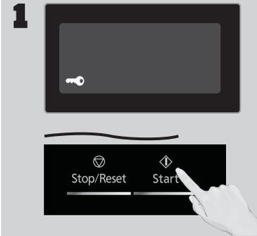
When the time of day appears in the display, press **Start** three times; "🔑" will appear in the display.
