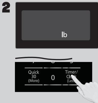
Press **Start** once, then Press **Timer/Clock (Less)** to cycle between the weight system, Metric (g/kg) or Imperial (oz./lb).
