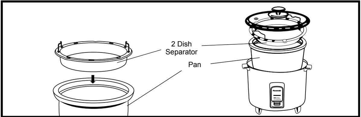
The 2 Dish Separator is a shallow pan, which can be placed on the Pan enabling you to cook 2 dishes at the same time. The figures above show you how to set the 2 Dish Separator.
