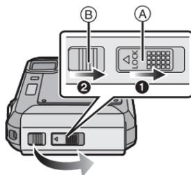
**2** **Battery:** Being careful about the battery orientation, insert all the way until you hear a locking sound and then check that it is locked by lever (C). Pull the lever (C) in the direction of the arrow to remove the battery.
