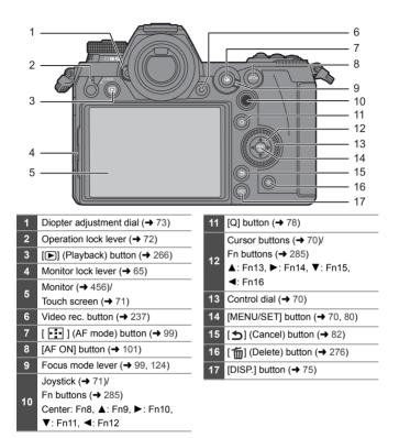
If you press [:☆:], the following buttons light. The lighting timing can be changed in [Illuminated Button] in the [Custom] ([Operation]) menu. (→ 344) – [[]) button/[[]] button/[[]] button/[[]]] button/[[]]
