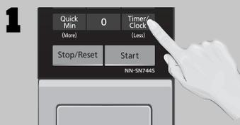
The start time can be delayed to start cooking at a later time. To do this, first press **Timer/Clock/Less**.
