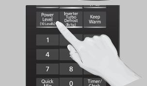
Press **Power Level** until the desired power level appears in the display. P10 is the highest and P1 is the lowest.
