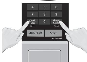
If desired, press **Quick Min/More** to add 20% more time than suggested. Press **Timer/Clock/Less** to subtract 20% cooking time.
