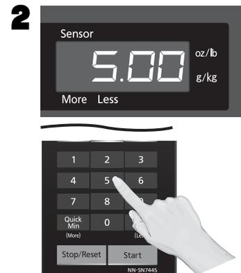
Set Cooking Time using the **Number** pads. P10 (HIGH) has max. cooking time of 30 minutes. For other power levels, the max. time is 99 minutes, 99 seconds.
