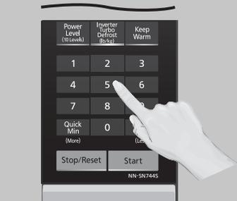
Set desired amount of time using **Number** pads (up to 99 minutes, 99 seconds).
