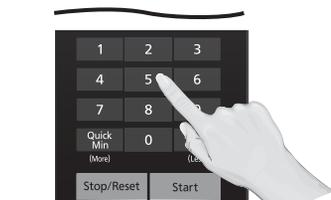
Set desired amount of stand time using **Number** pads (up to 99 minutes, 99 seconds).
