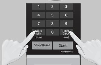
If desired, press **Quick Min/More** once to add 10 seconds or twice to add 20 seconds. Press **Timer/Clock/Less** once to subtract 10 seconds or twice to subtract 20 seconds.
