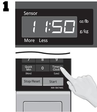
With the oven NOT cooking, press **Timer/Clock/Less** twice; the colon will blink. Enter time of day using the **Number** pads.
