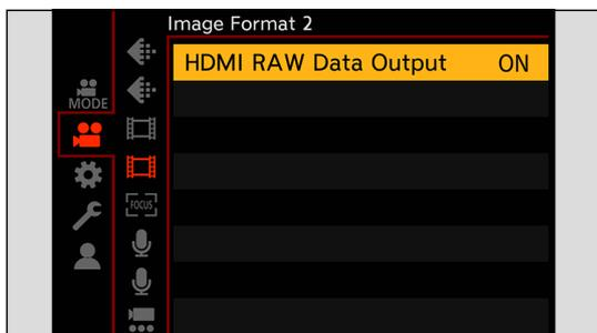
After setting [HDMI RAW Data Output] to [ON], display the menu screen with an SDI monitor or PC installed with “LUMIX Tether” and operate the camera.
