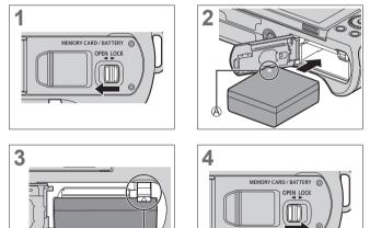
(A) Make sure to insert the battery in the correct orientation.
