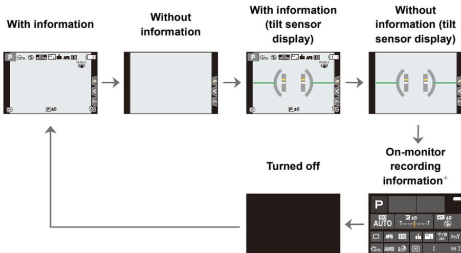
\* It is displayed when [Monitor Info. Disp.] in the [Custom] ([Monitor / Display]) is set to [ON]. You can touch the desired item and change its setting directly.
