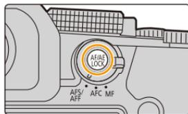
**3 While pressing [AF/AE LOCK], move the camera as you compose the picture and then press shutter button fully.**
