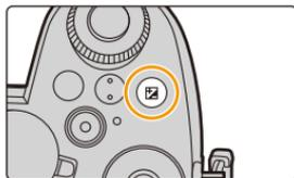
**2** Rotate the front/rear dial or the control dial to compensate the exposure.
