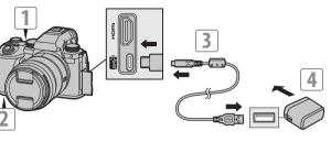
Approx. 220 min · Using the camera body and the supplied AC adapto
