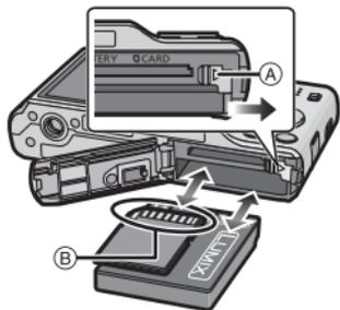
**Card:** Push it securely all the way until you hear a “click” while being careful about the direction in which you insert it. To remove the card, push the card until it clicks, then pull the card out upright.
