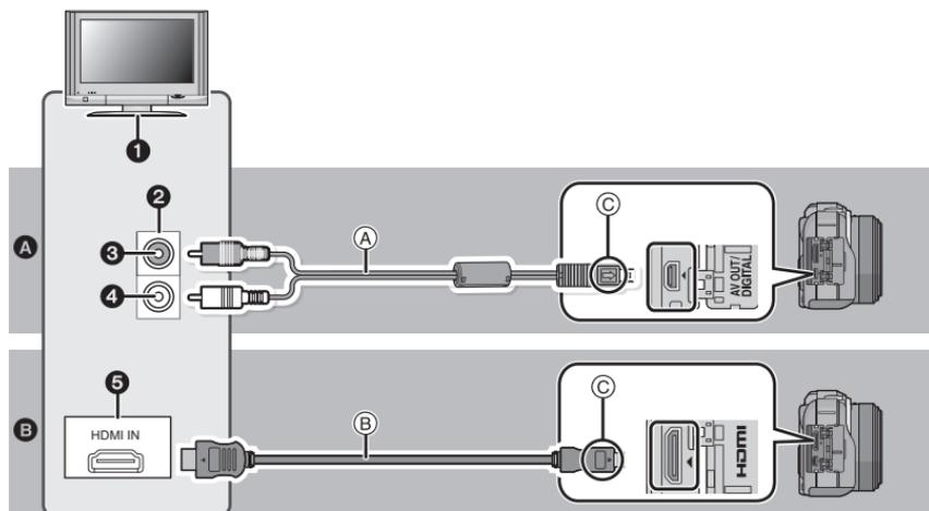
**A** To connect with an AV cable (supplied)
