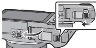
**2** **Battery:** Being careful about the battery orientation, insert all the way until you hear a locking sound and then check that it is locked by lever **A**. Pull the lever **A** in the direction of the arrow to remove the battery.
