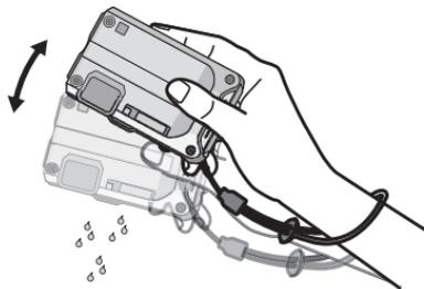
**3 Wipe off water drops on the camera with a soft, dry cloth and dry the camera in a shaded area that is well ventilated.**
