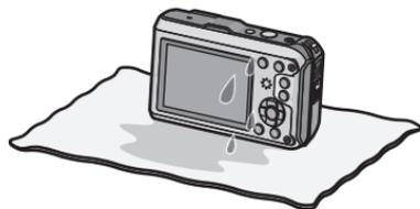
**4 Confirm that there are no water droplets, open the side door, and wipe off any water droplets or sand left inside using a soft, dry cloth.**
