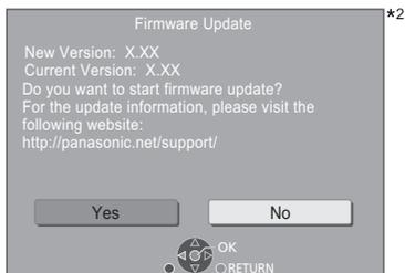
You cannot operate the unit until the update is complete. Don't remove the AC power supply cord during the update. Removing the AC power supply cord while the update is in progress may damage the unit.
