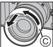
2 Align the mark **(B)** (◐) on the lens hood with the mark on the tip of the lens.
