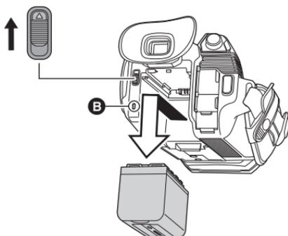
Move the battery release lever in the direction indicated by the arrow and remove the battery when unlocked.
