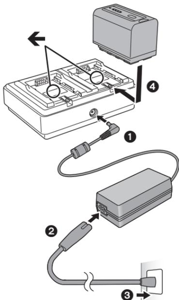
**1** Connect the DC plug of the AC adaptor to the DC IN 12 V connector of battery charger.
