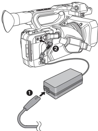
**1** Connect the AC cable to the AC adaptor and the AC outlet.
