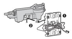
**2** Insert the hooks on the wall mounting adaptor into the holes (♠) and (♠) on the base unit.
