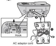
3 Insert the hooks on the wall mounting adaptor into holes **(A)** and **(B)** on the base unit
