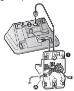
3 Insert the hooks on the wall mounting adaptor into holes ((2)) and ((3)) on the base unit.
