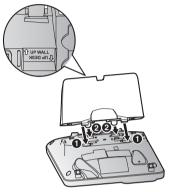
Mount the unit on a wall then slide down to secure in place.
