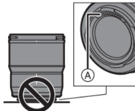
– Place the lens with its mount surface facing down.
