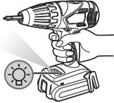
Before the use of LED light, always pull the power switch once.
