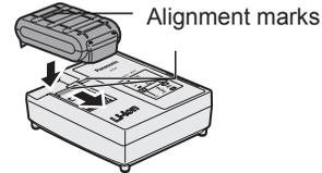
3. During charging, the charging lamp will be lit. When charging is completed, an internal electronic switch will automatically be triggered to prevent overcharging.
