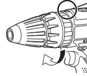
If the clutch handle cannot be set at "drilling" or "hammering" mode after drilling with clutch function, set the clutch handle at position 1 and operate the clutch for a second.
