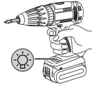
Before the use of LED light, always pull the power switch once. Press
