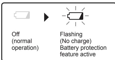
Excessive (complete) discharging of lithium ion batteries shortens their service life dramatically. The driver includes a battery protection feature designed to prevent excessive discharging of the battery pack.
